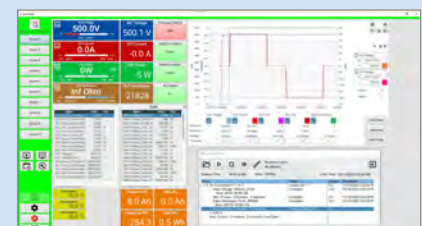
Results display screen showing voltage, current, and the results of a capacity simulation test.
